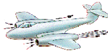
A jet engine accelerates a small volume of air by a large amount
