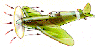
A propeller accelerates a large volume of air by a small amount
