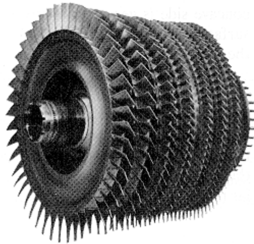
An axial flow compressor (stators omitted for clarity). This is the high pressure compressor from a General Electric F404 engine.
